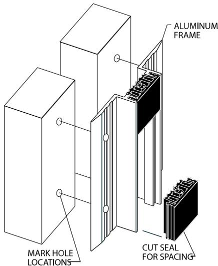
1. Install the architectural joint system on a level wall surface. Additional shims may be required to raise the tops of the frames.
