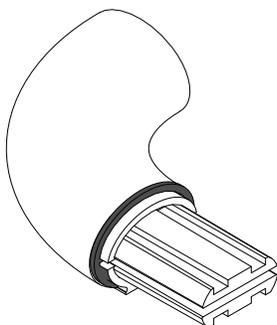
2. Attach Returns and Corners to retainer, leaving 1/16" [2mm] gap between Return/Corner and retainer allowing for adjustment. See Fig. 3.
