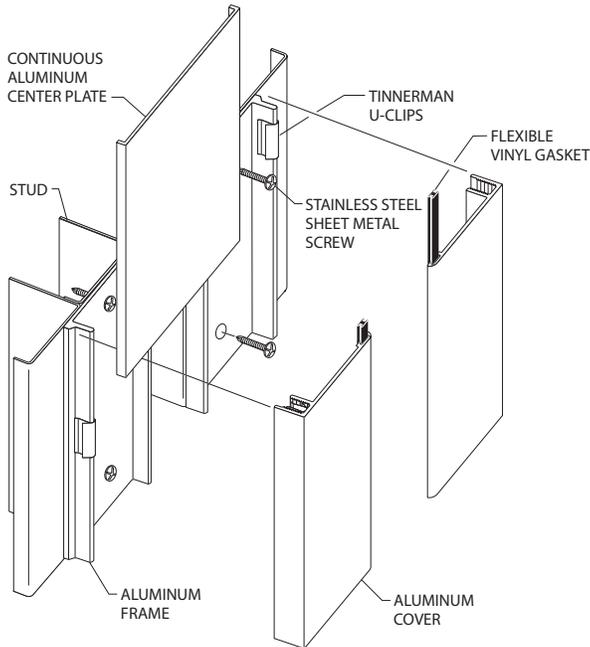
1. Install the architectural joint system on a level surface, making sure the tops of the aluminum covers align with the finished height of the  $\frac{5}{8}$ " drywall. Shims may be required to raise the tops of the frames.
