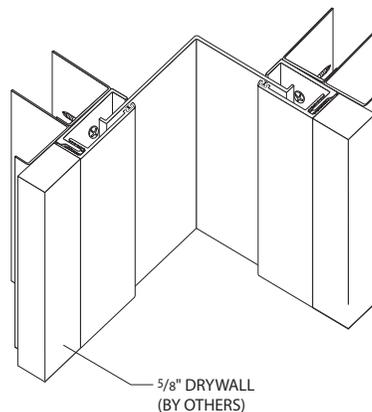
Fig. 2b (300-A09 completed installation)
